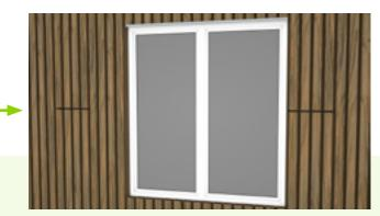
1. For shallow window or door reveals it may be possible to just use the L corners on the two verticals either side of the window. At the base of the window an L corner can be used only if there is not an existing sill is in place. Ensure adjoining corners are mitre cut for best finish.
