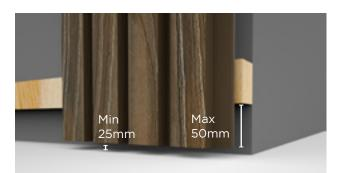
**\*NOTE:** Locate the first joist to ensure a clearance of at least 25mm can be left between the bottom of the cladding plank and the ground surface. The cladding plank should not overhang the bottom joist unsupported by more than 50mm
