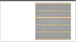
2. Supporting joists (not supplied) should be a minimum of 25mm deep and 38mm wide. Fix joists to the wall at maximum of 450mm spacing with relevant anchor fixings.
