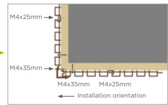
1. Install L Corners vertically at external corners using high quality adhesive sealant and 35mm long colour head screws spaced at 900mm centres.
