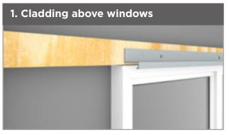
1. When cladding above windows or doors, a colour coded steel drip trim should be installed to the joist to carry water away from the building. Cut the trim to the width of the window and fix it using 25mm screws prior to installing any cladding. The spacing between screws should be 300mm maximum.
