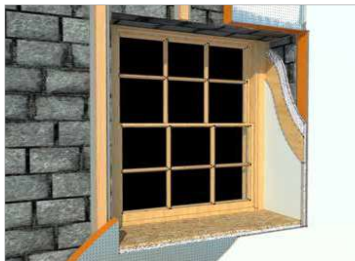
Image showing Spacetherm WRB applied internally to a reveal on an existing external wall structure.
