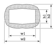
CR Ducts are made of compressed glass wool with inner & outer surfaces covered by a layer of CR Foil.
