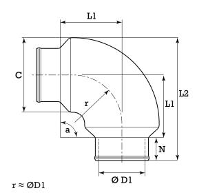
CR Bends are made of compressed glass wool with inner & outer surfaces covered by a layer of CR Foil.
