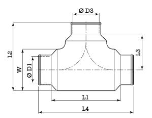
CR T-pieces are made of compressed glass wool with inner & outer surfaces covered by a layer of CR Foil.
