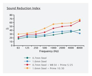
INS Acoustics have recognised the complex problems associated with noise breakout from ductwork and have developed performance data from laboratory test results.
